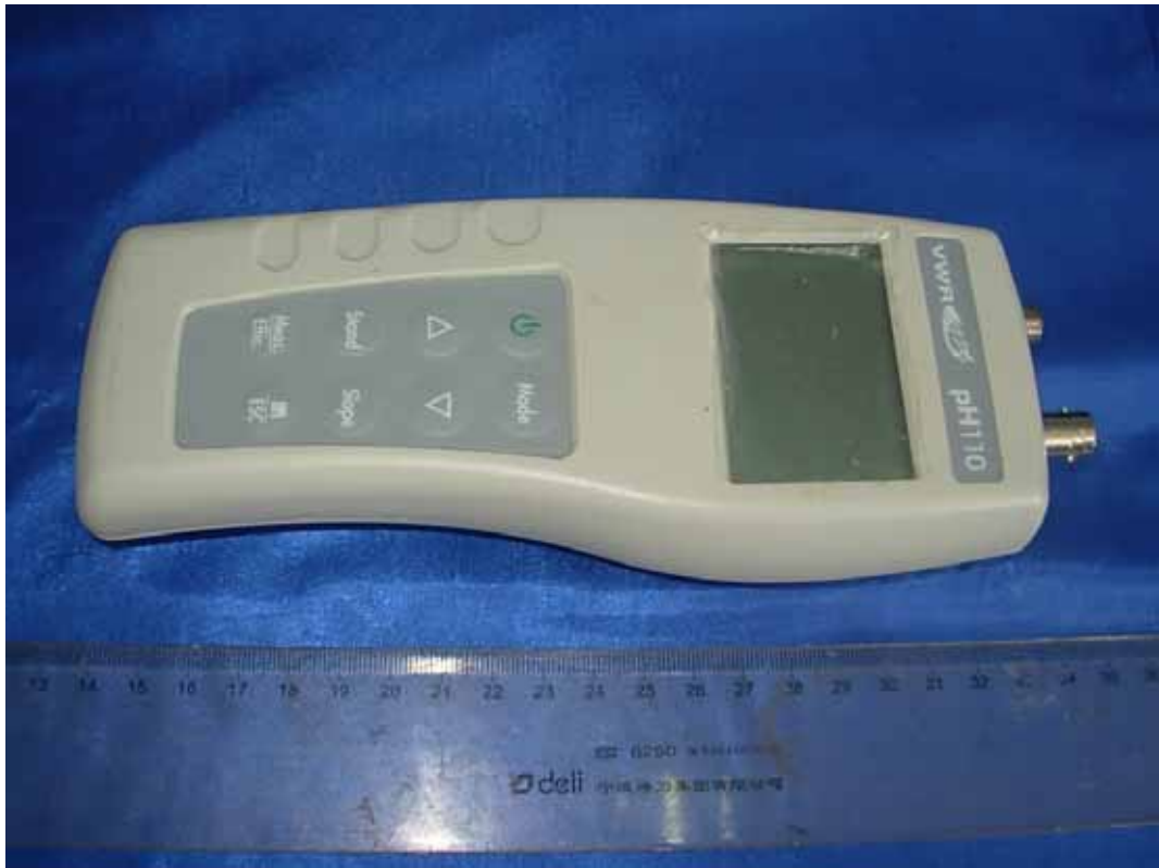
FIGURE 10 PORTABLE pH, mV AND TEMPERATURE INSTRUMENT (M/N: PH110) GENERAL APPEARANCE (FRONT VIEW)
