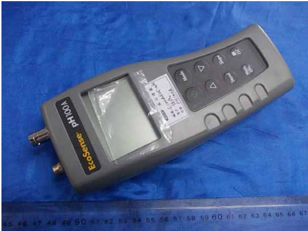
FIGURE 2 PORTABLE PH, MV AND TEMPERATURE INSTRUMENT (M/N: PH100A) GENERAL APPEARANCE (FRONT VIEW)
