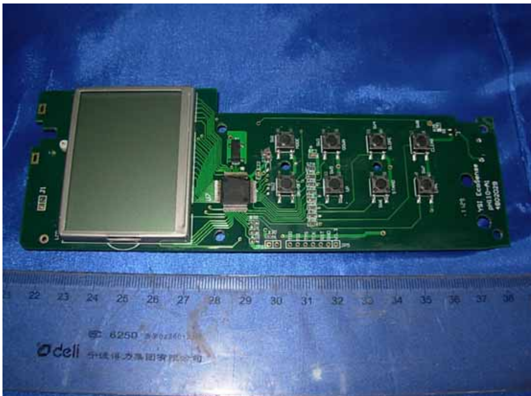
FIGURE 8 PORTABLE PH, MV AND TEMPERATURE INSTRUMENT (M/N: PH100A) MAIN BOARD (SOLDERED SIDE)
