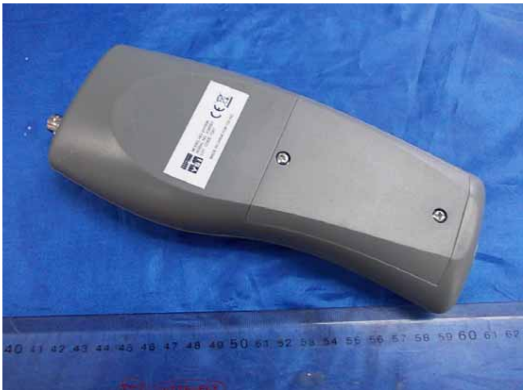
FIGURE 3 PORTABLE PH, MV AND TEMPERATURE INSTRUMENT (M/N: PH100A) GENERAL APPEARANCE (BACK VIEW)
