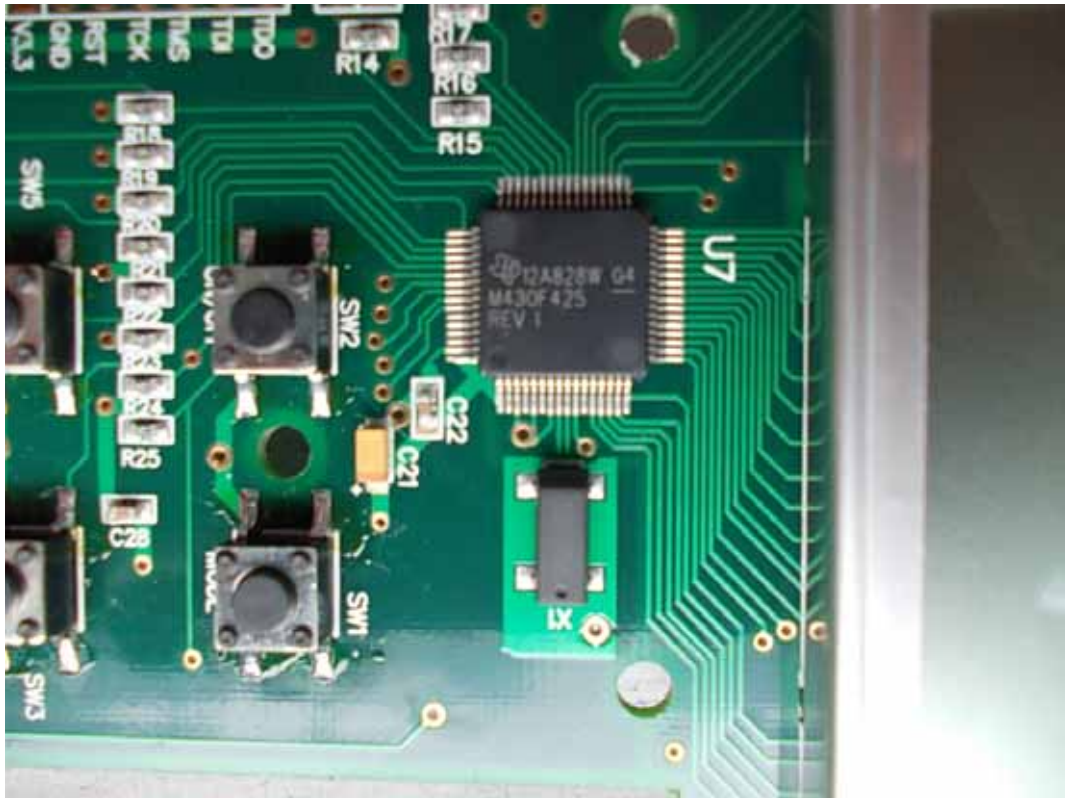
FIGURE 9 PORTABLE PH, MV AND TEMPERATURE INSTRUMENT (M/N: PH100A) CHIP ON MAIN BOARD
